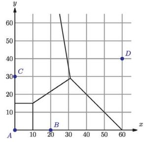
Using a Voronoi diagram: The vertices of the regions are points of maximal local distance from adjacent towns; the one furthest from all is at the *BCD* vertex.
