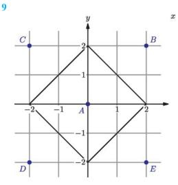
On the Voronoi diagram of the town, the cell containing A is a square of side  $\sqrt{8}$  so has area 8 km<sup>2</sup>.
