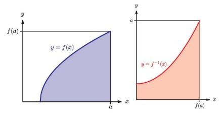
where af(a) is the area of the rectangle bordering the limits of the integral area, which would have vertices at the origin, (0, f(a)), (a, 0) and (a, f(a)).
